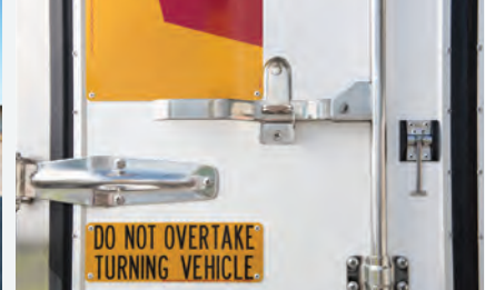
GALVANISED STEEL EXTERNAL LOCK-ROD DOOR HARDWARE
